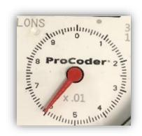
**Sweep Hand Dial** – This dial shows the rate of water that is passing through the meter at the moment. The sweep hand can be used for leak detection. One rotation of the sweep hand represents 0.1 (1 tenth) gallon being used at that moment. If all water in the building is turned off and the sweep hand is still spinning on the meter, water is still flowing through the meter. Since all water is turned off, there must be a leak somewhere in your system.
