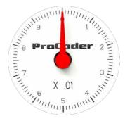
Atypical ProCoder sweep hand contains 10 large ticks numbered 0-9. Between each large tick, there are 9 small ticks numbered .1 - .9. Depending on the size and meter type, a multiplier will also be present and located below the red hand. Let's demonstrate how to read the sweep hand.
